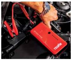
3 Locate the battery and connect first the red clamp (+) to the positive terminal, then the black clamp (-) to the car frame or to the negative terminal of the battery.
